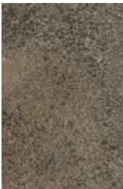
Water based acrylic paint without VpCI® additive.
